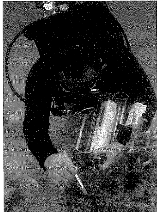
Figure 3. The submersible pulse modulator (PAM) or Diving-PAM (Walz, Germany) used for photosynthetic measurements of coral colony.
